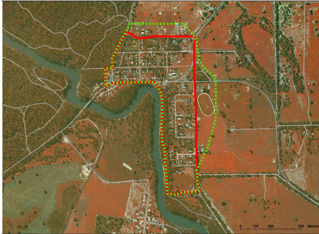
■ Figure 5-1 Proposed levee alignments for Barmah township flood mitigation (alignment 1: red solid line; alignment 2: green dotted line)
